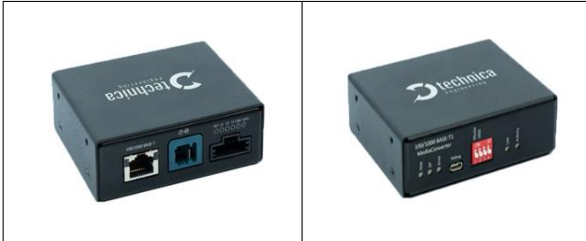
Figure 1-1: 100/1000BASE-T1 MediaConverter MATEnet
