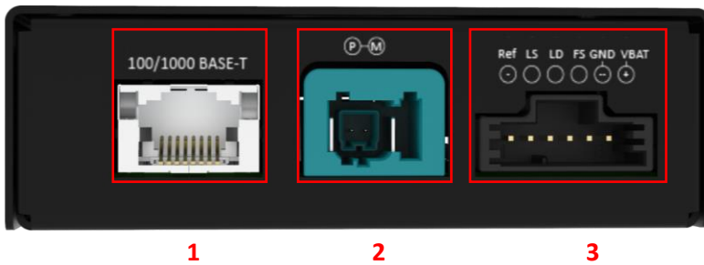
Figure 2-2: Backside of MediaConverter
